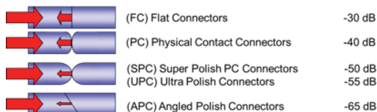
Figure 5. Typical connector types and reflectance values
